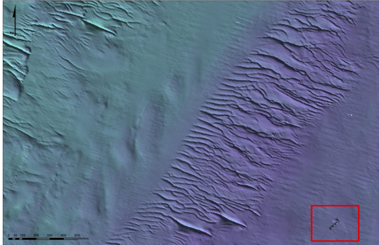
Above the location of the SS Atxeri Mendi from shaded relief imagery acquired during Infomar survey CV12_02 Irish Sea area and below an image of the SS Atxeri Mendi at 50cm resolution.
