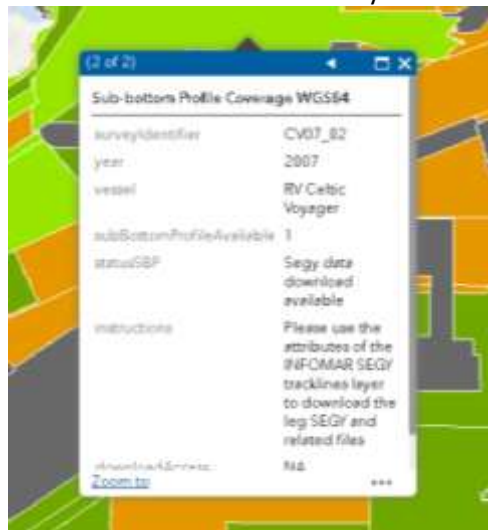
Figure 7 - shows a light green polygon pop up from the 'Sub Bottom Profile Availability' layer Orange polygon means that the data has not yet been converted to SEG-Y. This means, depending on the vessel, it will either be available in *.COD, *.JSF or *.RAW. This data needs to be requested from data@infomar.ie
