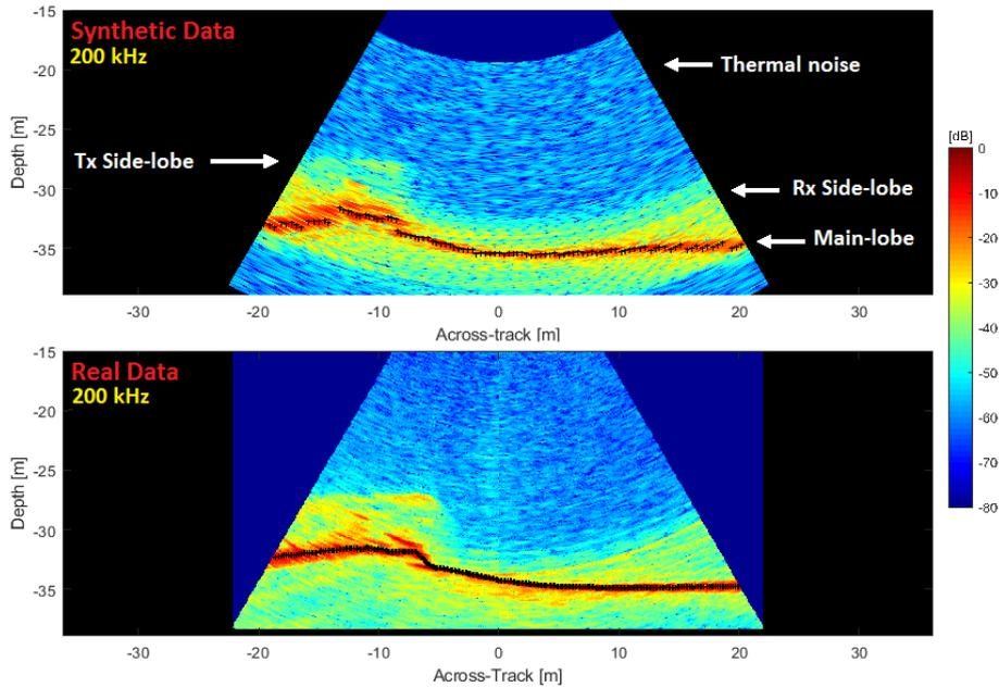
Fig. 2: Scenario 1: Upper: simulated water-column data. Lower: Real water-column data. The black markers “+” indicates the detected sea bottom.
