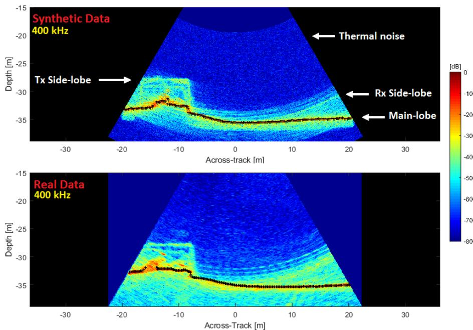
Fig. 3: Scenario 2: Upper: simulated water-column data. Lower: Real water-column data. The black markers “+” indicates the detected sea bottom.
