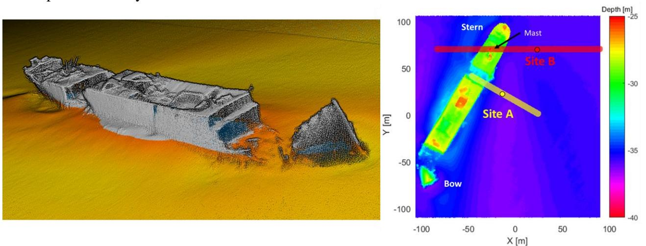
Fig.1: Left: Point Cloud generated from the multi-settings survey data.
