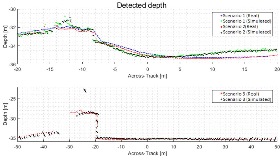
Fig. 5: Estimated depth after bottom detection. For real data the depth was estimated via the constructor bottom detector with minimum depth mode.
