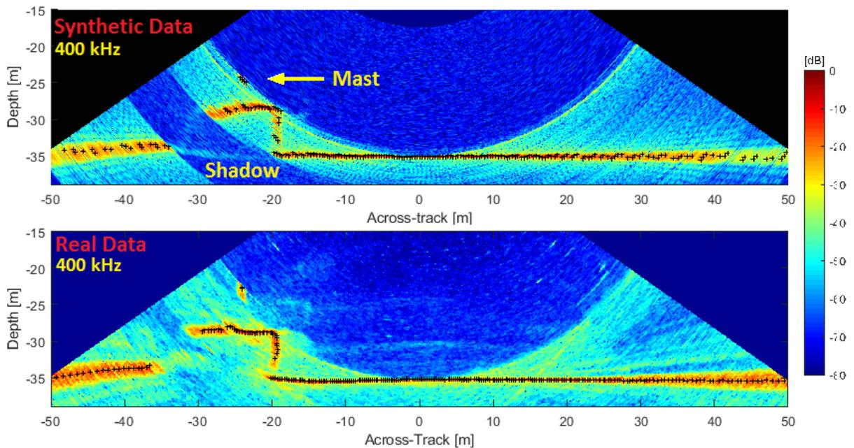
Fig. 4: Scenario3: Upper: simulated water-column data. Lower: Real water-column data. The black markers “+” indicates the detected sea bottom.
