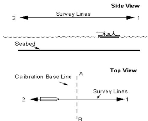
**Figure 6.** Testing for roll bias.
