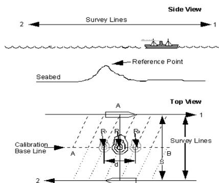
Figure 7. Testing for yaw roll bias.
