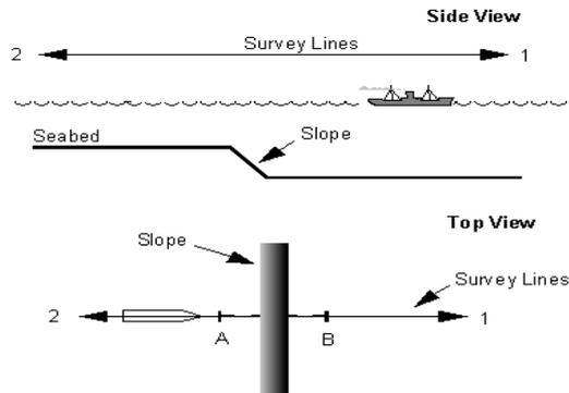
**Figure 5.** Testing for pitch bias.
