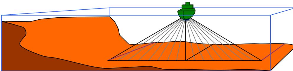
**Figure 1.** Swath sounder sonar system swathe.
