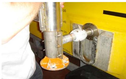
**Figure 2.** Example of a keyed pole mount.
