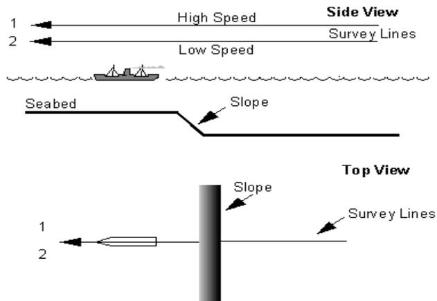
**Figure 4.** Testing for latency.
