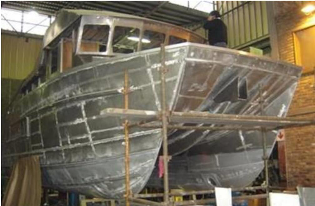
Near complete fabrication of aluminium external structure of RV Keary with bridge under construction.
