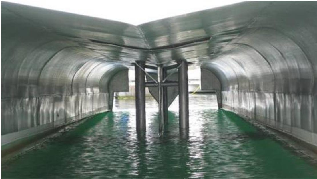
View of extended pod and hydrofoil which allows RV Keary to transit efficiently between survey areas and port.
