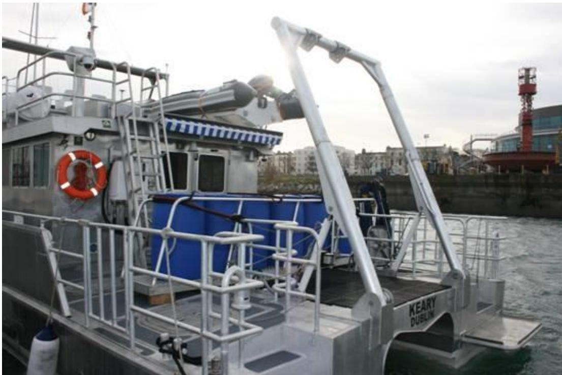
Back deck of RV Keary with A-frame used when performing seabed sampling operations.
