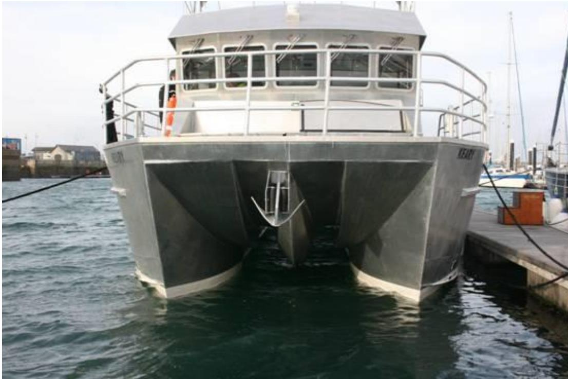
View of the bow of RV Keary with wave piercer in the centre to minimise the effect of waves on the vessels stability which improves data quality and comfort.
