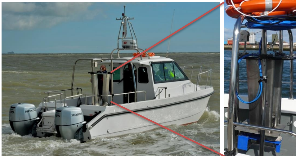
R2Sonic Multibeam Sonar mounted on hydropod system
