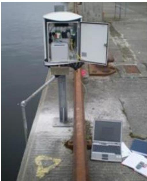
An OTT Nimbus gauge at Rossaveal, Co. Galway. The battery, data logger and air pump are all housed in a water proof box on the pier.
