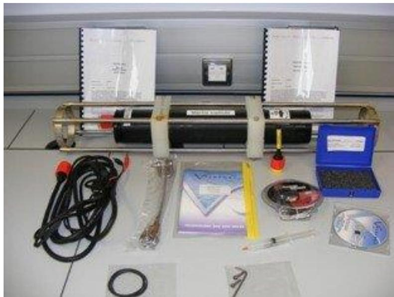
Midas WLR tide logging instrument used to measure changes in offshore tide height during the survey.
